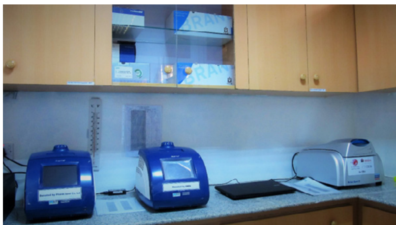
Conventional and real-time PCR machines
