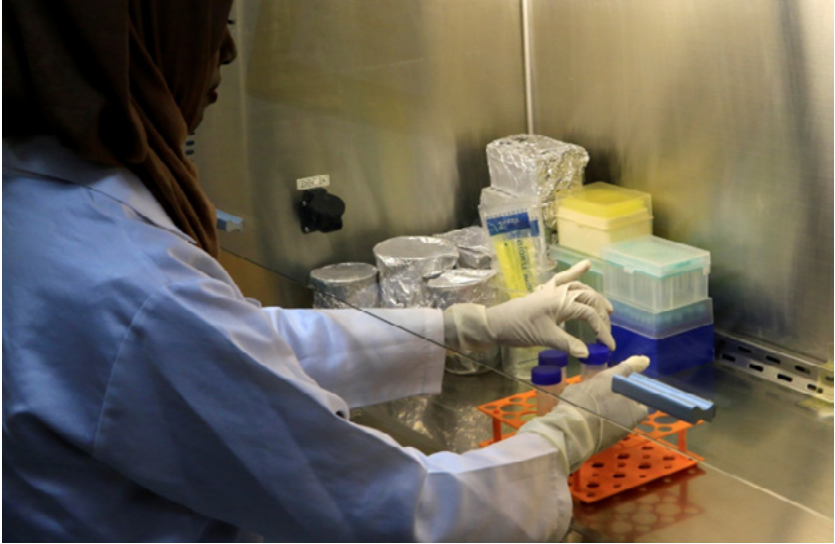
Working within the Class II Biological Safety Cabinet
